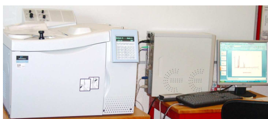
GC (PerkinElmer Clarus 400) equipado com detector FID (Waltham, USA) Coluna capilar BP 20 (30 m x 0.32 mm I.D. x 1.0 µm film thickness; SGE, Australia)
